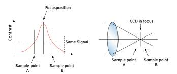
be at a lower level than on the CCD but of the same value at each sample point. If the focus were incorrectly adjusted then the contrast measured at the sample points would not be equal. Thus it is possible not only to find the sharpest focus position but also the direction of any necessary adjustment required when focus is not sharp.
